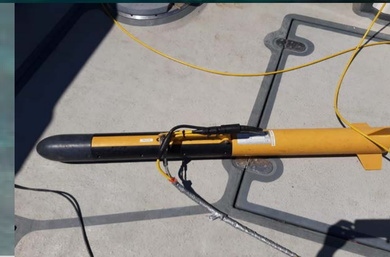
Figure 1 (Right) The Side scan Sonar Tow Fish used. Figure 2 (Left) A map of the Special Area of Conservation surrounding Plymouth sound and surrounding estuary.
