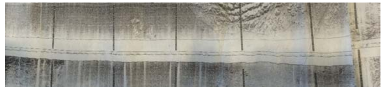
Figure 6: An example of the side scan sonar read out used to construct the map
