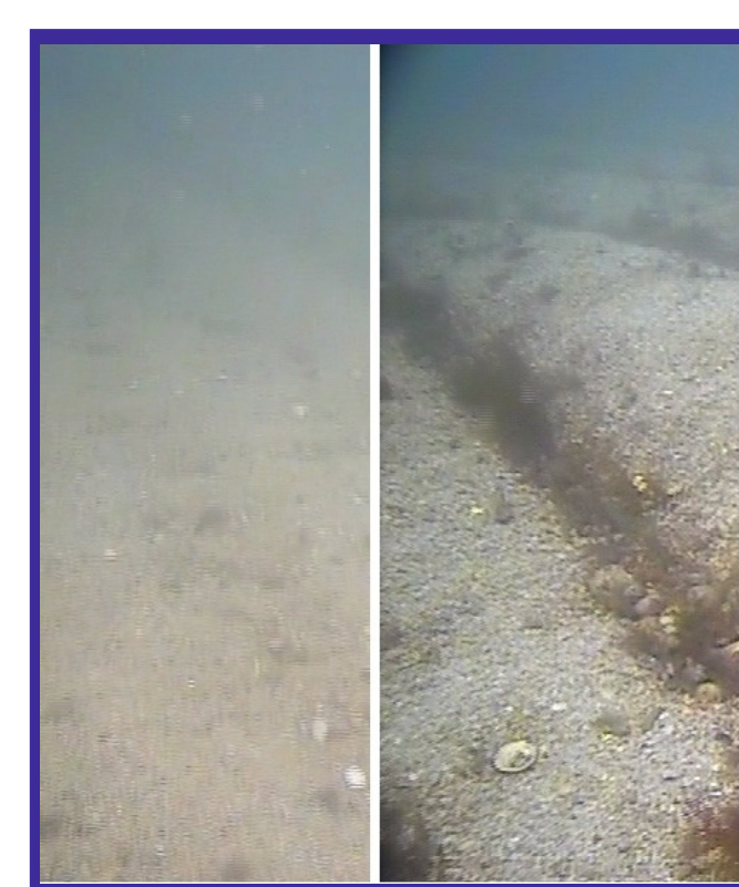
FIG. 1 shows change in bedforms on the sea floor. The image to the left shows an area where the seabed is flat and current speed is lower. The image to the right shows an area where ripples dominate and current speed is higher. The majority of the sea floor seen on the video has similar bedforms to those seen on the right. In the rippled areas fauna and flora tend to live in the troughs of each ripple.
