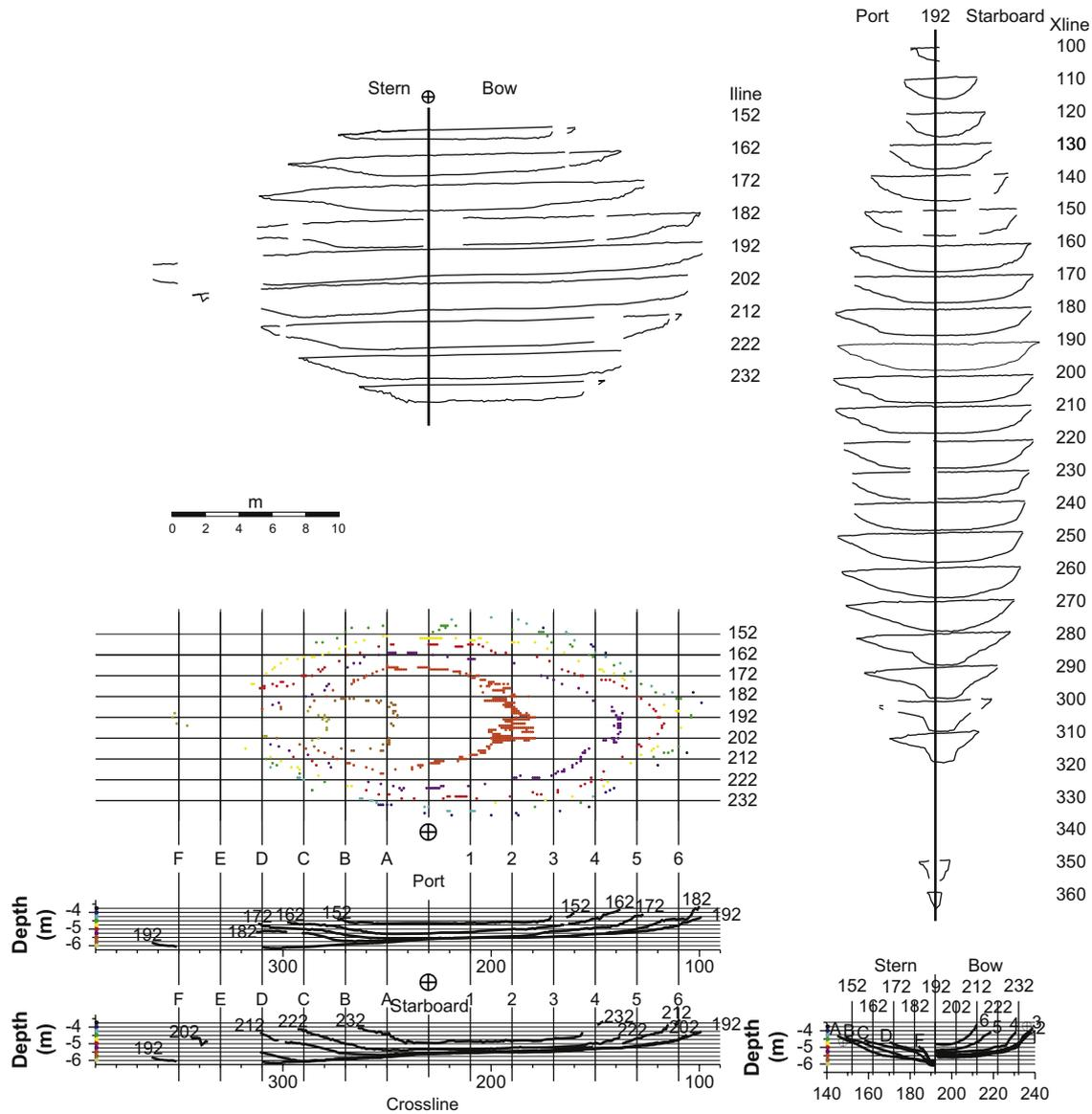
Fig. 13. Body plan of the buried remains of the *Grace Dieu*, derived from the 3D reconstruction.
