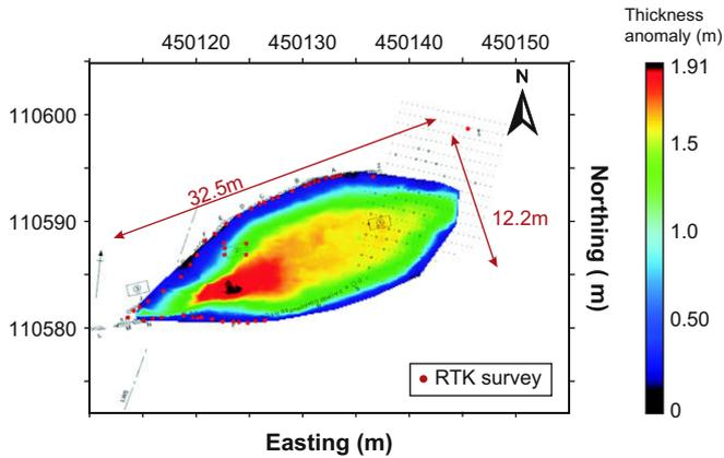
Fig. 11. Isopach map showing the thickness of the anomaly (in metres) and comparison with the terrestrial RTK data and excavation plan (Clarke et al., 1993).
