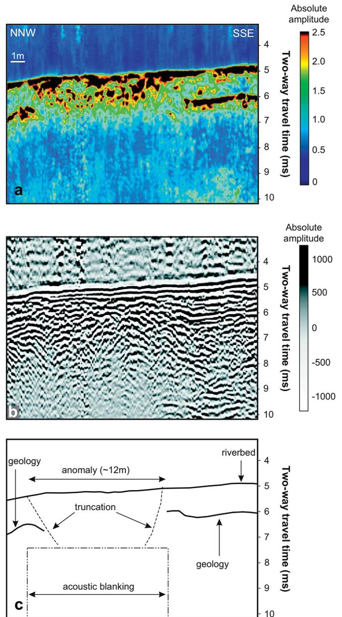
Fig. 5. Typical vertical section acquired over the wreck site (Line 183 indicated in Fig. 4). (a) Enveloped correlated data, (b) raw correlated data and (c) acoustic interpretation.
