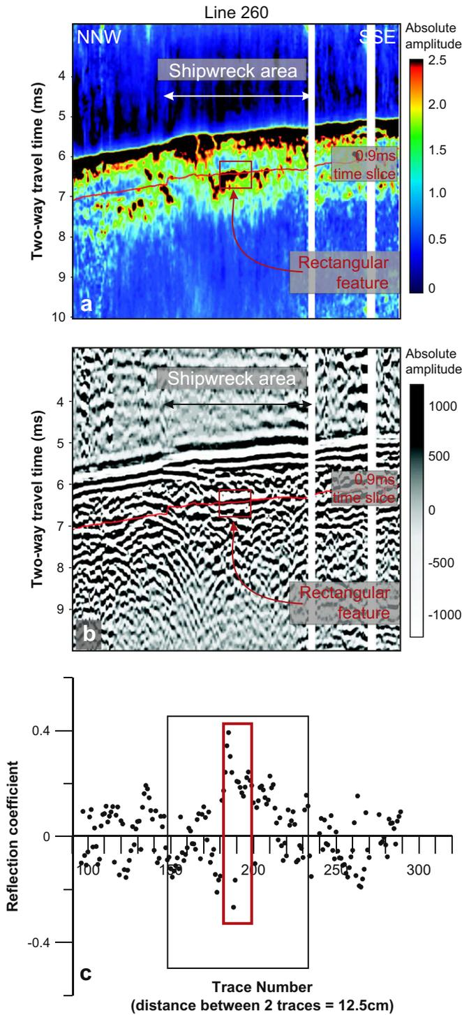
**Fig. 9.** Reflection coefficient calculation for line 260 (see Fig. 6). (a) Correlated, enveloped data; (b) correlated, raw data; and (c) reflection coefficients along the line at a depth of 0.9 ms. Black box indicates position of the shipwreck, red box indicates position of the rectangular feature; colour bar represents absolute amplitudes.
