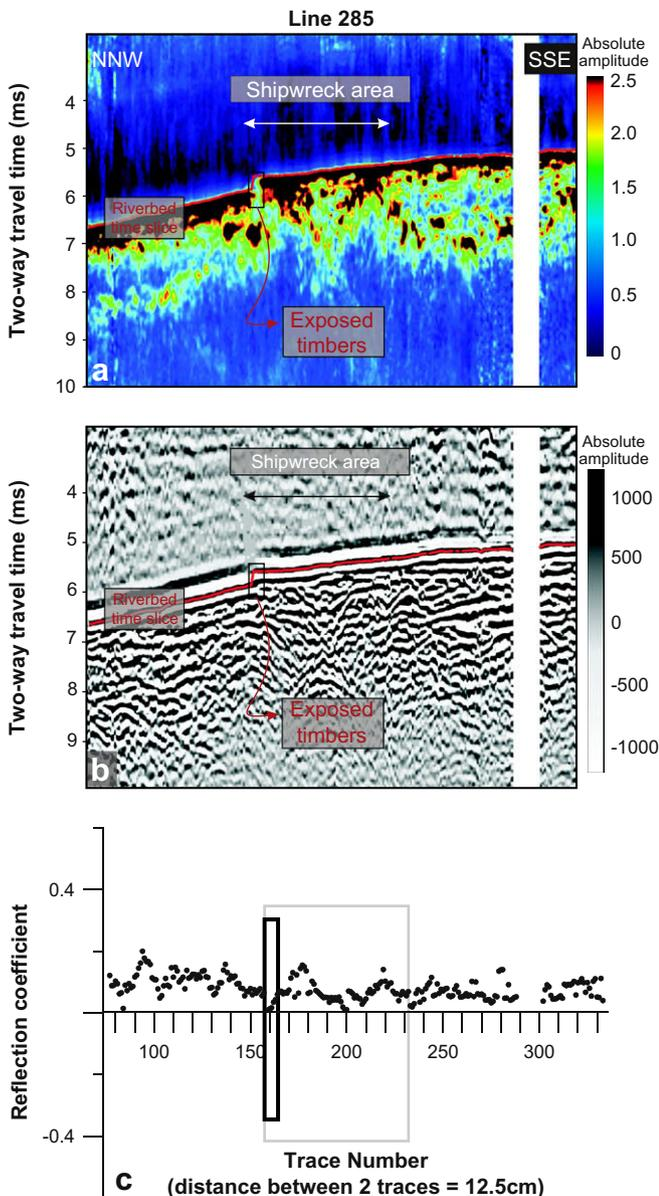
Fig. 7. Reflection coefficient calculation for line 285 (see Fig. 6); (a) Correlated, enveloped data; (b) correlated, raw data and (c) reflection coefficients along the line for the riverbed. Back box indicates position of the exposed timbers; grey box indicates position of shipwreck; colour bar represents absolute amplitudes.
