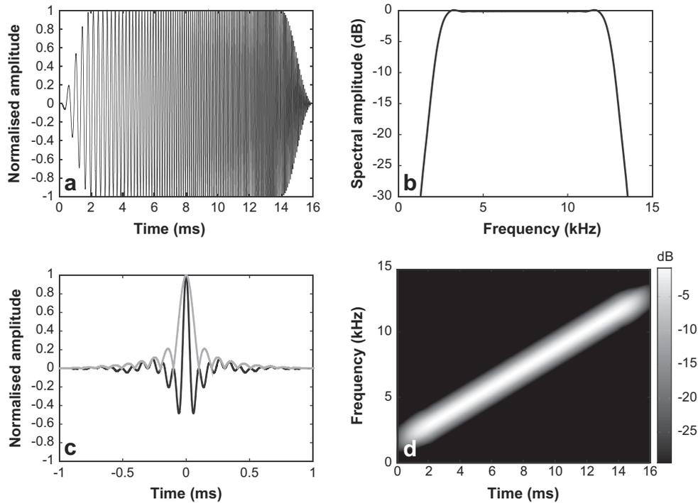
**Fig. 3.** Source sweep. (a) Time domain representation showing sine-squared 8th sweep. (b) Power spectrum of 1.5–13 kHz pulse. (c) Klauder wavelet, the normalized auto-correlation function of the sweep, with its envelope. (d) Spectrogram showing linear frequency function (dB scale).
