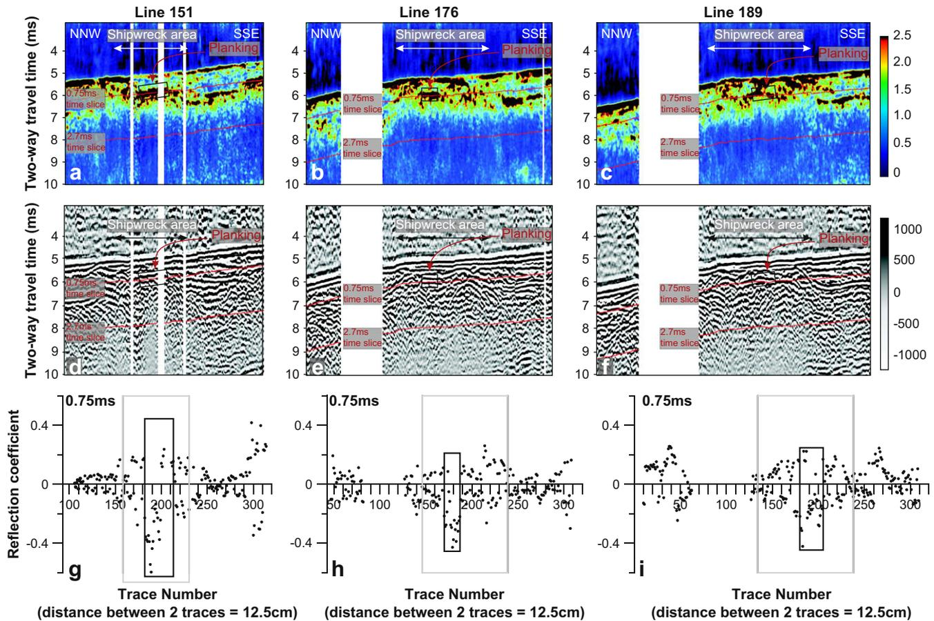
Fig. 8. Reflection coefficient calculation for lines 151, 176 and 189 (see Fig. 6). (a–c) Correlated, enveloped data; (d–f) correlated, raw data; (g–i) reflection coefficients along the lines at a depth of 0.75. Black box indicates position of possible buried planking, grey box indicates position of shipwreck; colour bar represents absolute amplitudes.
