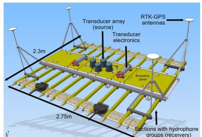
Fig. 2. Survey equipment configuration; high-resolution 3D Chirp system.
