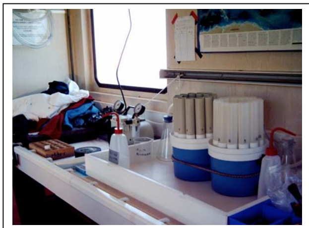
Fig. 12.2 Two x 12 port filtration rigs for ^{14}\text{C} filtering in the RN container
