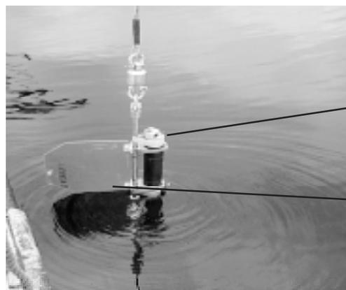
Three orthogonal acoustic transducers for u,v,w
