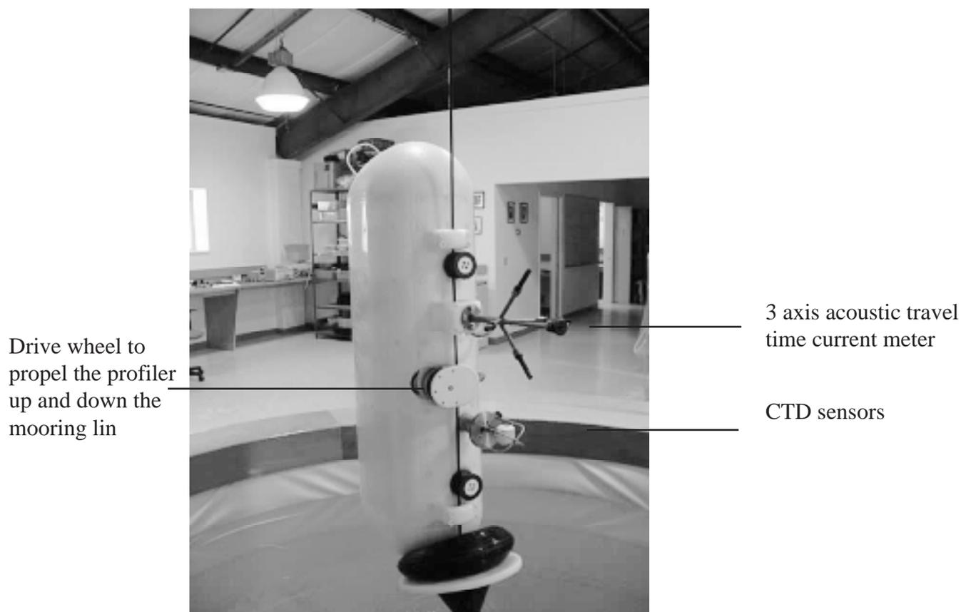
Figure 3 Acoustic travel time current meter as one instrument among many on a package capable of crawling up and down a wire mooring to obtain profiles of properties in water depths of up to 5000 m. Illustration courtesy of McLane Research Laboratories.
