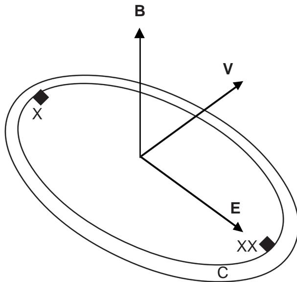
Figure 2 Sketch showing the Faraday effect, which forms the basis of the electromagnetic current meter. The effect results in a potential difference  $E = B V L$  induced between two electrodes ( $X$  and  $XX$ ) with a separation  $L$  when a conductor (seawater) moves at a resolved velocity  $V$  perpendicular to the line  $X - XX$  and perpendicular to a magnetic field with a flux density of  $B$  induced by coil  $C$ .
