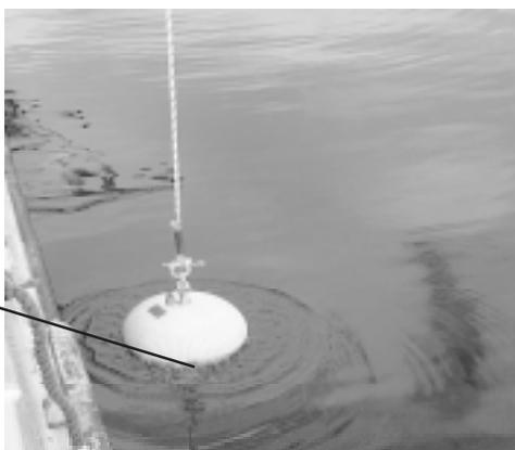
Four electrodes spaced at 90° on the equator
