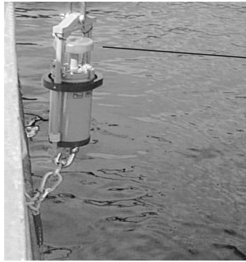
Two-axis acoustic transducer
