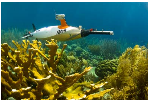
The AUVs were capable of precision mapping of benthic habitats with good depth holding and terrain following
